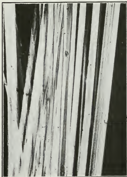
Fibre from the Carolina district, Transvaal. Magnified 200 diameters.
